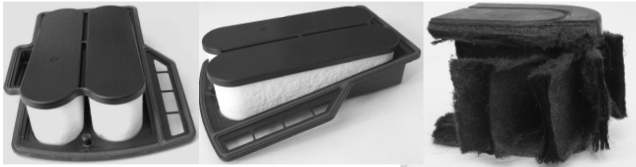
Fig. 8. New filter coalescer – two left photos, and a section of a coalescer taken for lab inspection after long operation on an engine (layers of fibers separated in the laboratory for detail study) – right photo
